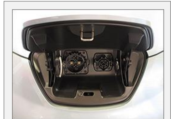
The standard J1772 receptacle (right) can receive charge from Level 1 or Level 2 equipment. The DC fast charge receptacle (left) uses a different connector.
