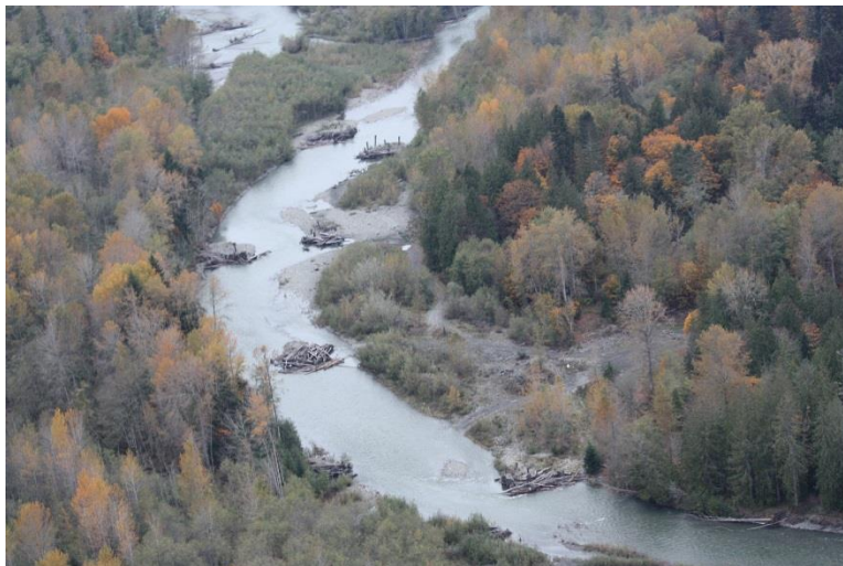
Figure 4 – Example of Engineering Log Jams in the Elwha River, WA (USBR and ERDC 2016)
