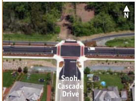
*This photo shows the intersection after construction. Snohomish Cascade Drive is the first raised, tabletop intersection in Snohomish County.*
