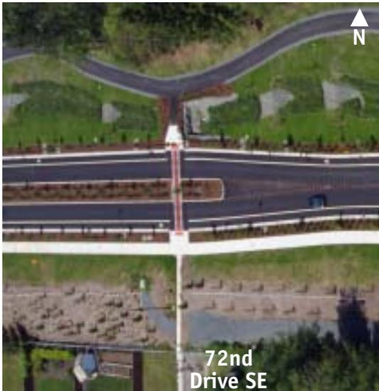
*In response to input from residents, the plan for vehicle access was eliminated at the 72nd Drive SE stub. The final design provides pedestrian-only access to Puget Park Drive at this location.*
