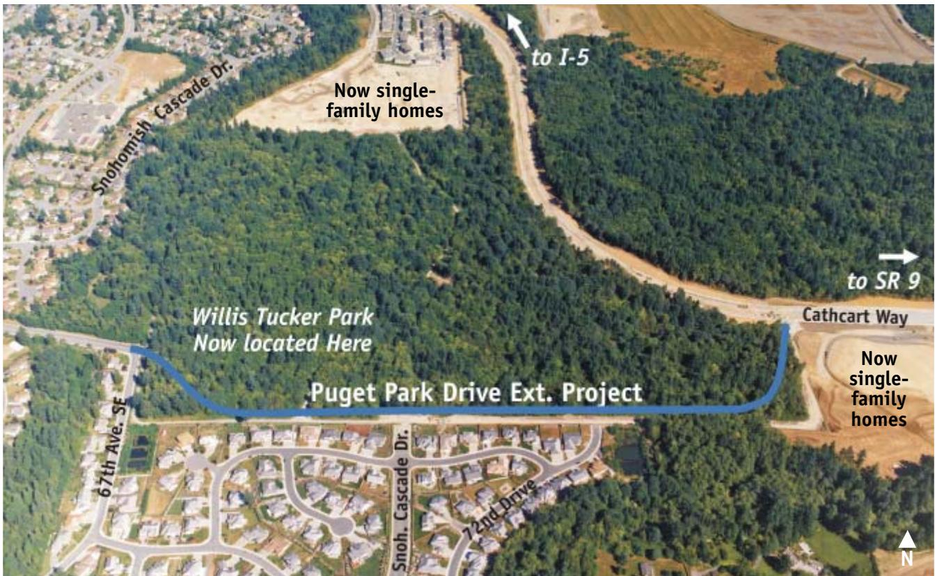
The project extended Puget Park Drive from 67th Avenue SE to Cathcart Way. A right-turn in and right-turn out intersection was created at 67th Avenue SE. A tabletop intersection was constructed at Snohomish Cascade Drive.
