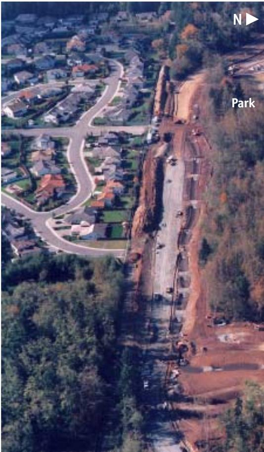
*Stormwater runoff filters through 13 rain gardens (shown here on the right side of the road).*
