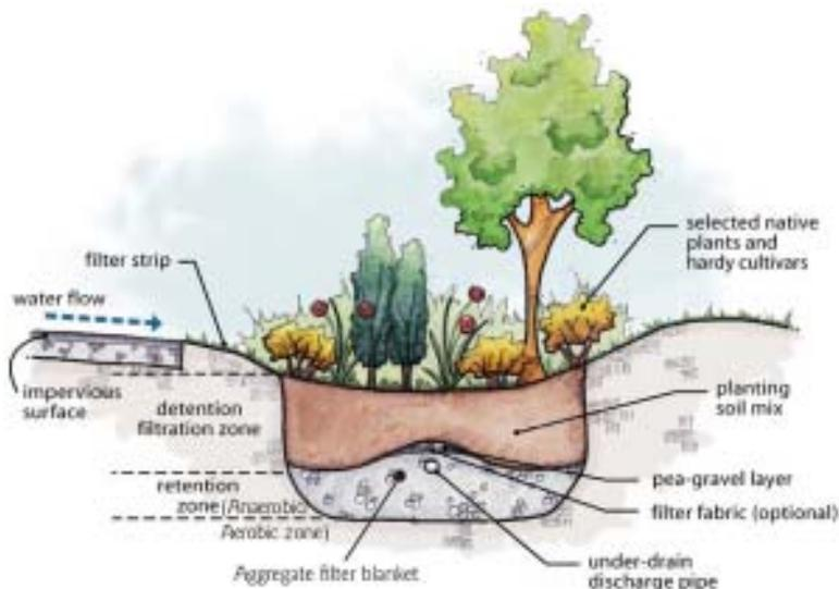
A series of 13 interconnected rain gardens, totaling approximately 1,600 linear feet, were ultimately incorporated into the design, with each swale cascading into the next. The soil types at this site infiltrate only a small portion of runoff naturally. The rain gardens slow runoff and allow additional infiltration.
