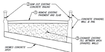
Schematic Section of 1920 Arch
